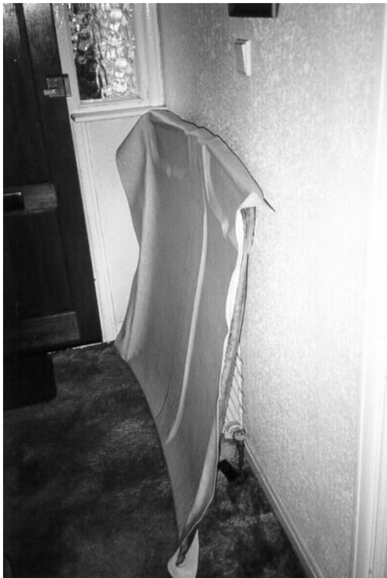
Headlining panel being warmed over radiator
