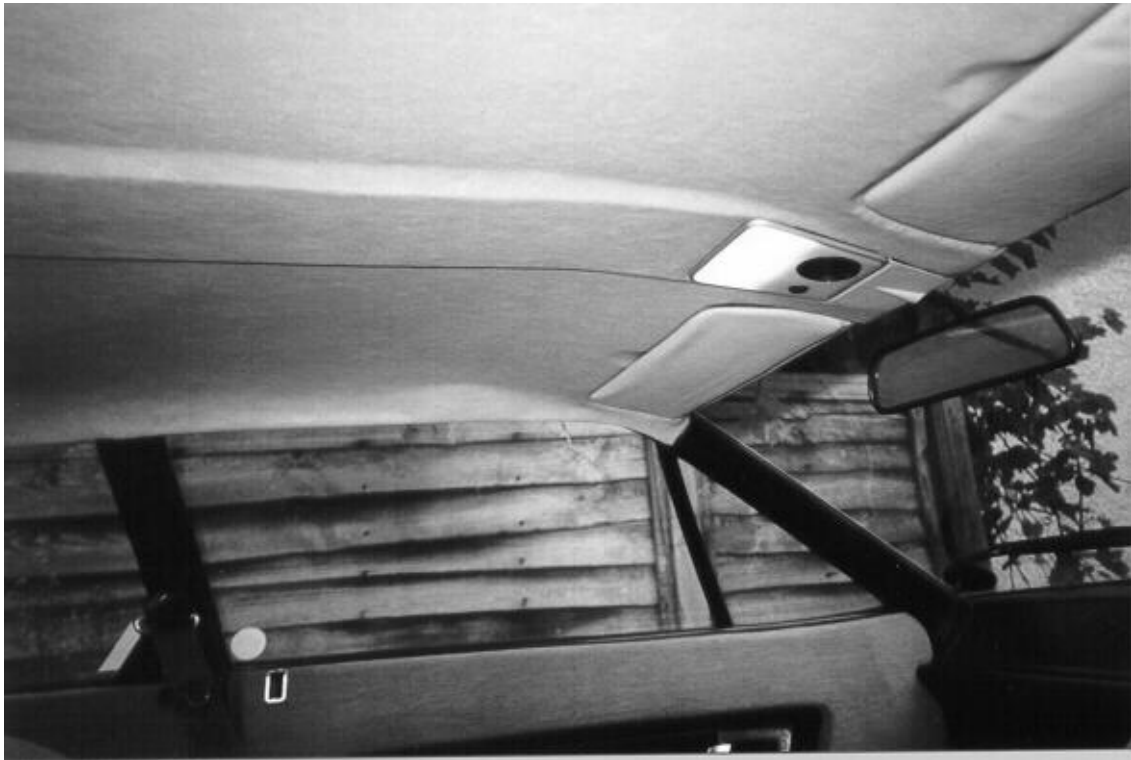
Front view of headlining complete with 'dimples' to lower the sunvisors
